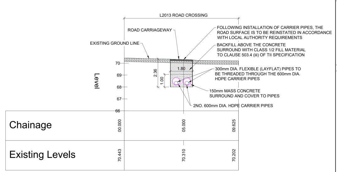
SECTION 3 CH0.0M TO 9.6M SCALE H 1:100 , V 1:100, DATUM:66.000
